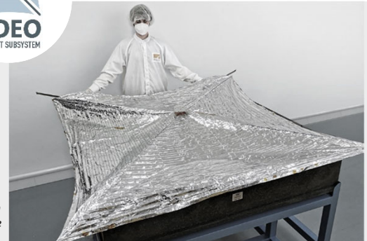
ADEO-N deployed demonstration model with sail size 3.6 m 2
