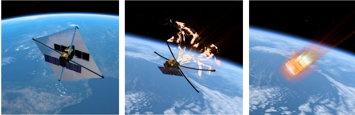
Deployment after mission time Deceleration until dense atmosphere Burn of satellite in dense area
