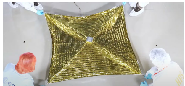
Deployment Sequence ADEO-N (snapshots of a movie)
